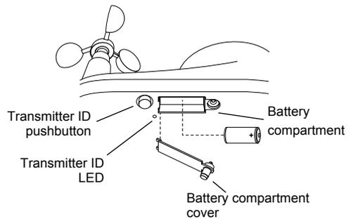
To verify power, wait 30 seconds then push and release the white transmitter ID pushbutton next to the battery compartment. The green transmitter ID LED next to the battery compartment will illuminate when you press the pushbutton.
