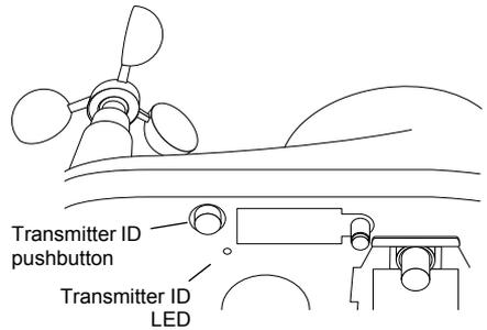
Unless you have intentionally changed your transmitter ID, the LED should blink *one time* because the default transmitter ID for the ISS is "1." If you have changed the ID, the LED should blink the number of times equal to the ID you have set (i.e., twice for an ID of '2,' three times for an ID of '3,' etc.).
